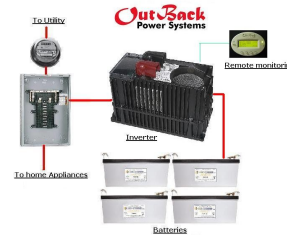
battery backup system
